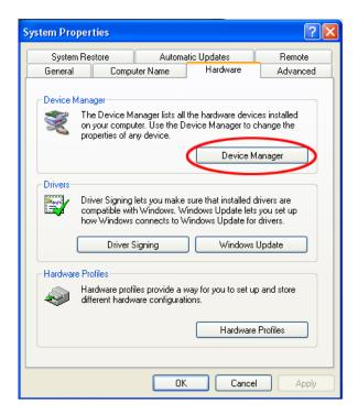
Find [COM and LPT] port in [device manager], click the plus sign on the left, record serial interface name that computer provides, as following chart, the serial port is COM1.
