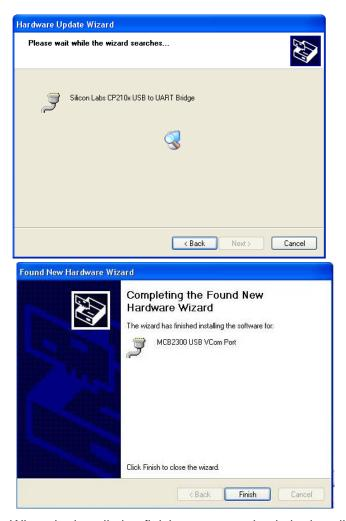
When the installation finish, can go to check the installed COM port inside the device management, as following image shows:
