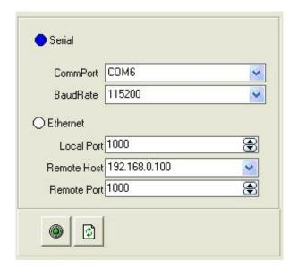
Press to start communication, when there is green point in the right down corner showing on the software, it means the communication is ok, and you can use the software to control the device now, the software operation is the same as VSP 198CVS.
