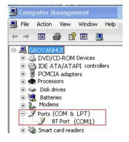
Remember the COM you are using and then run the control software, find
