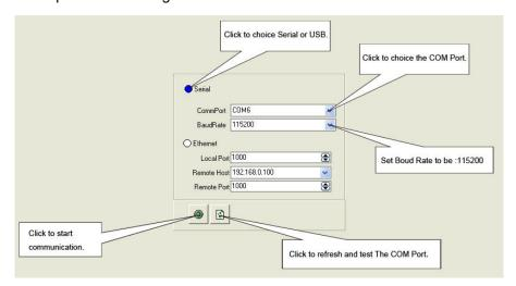
For more detailed information, please refer to: "How to Connect Windows Control Program by RS232 Interface". User can also connect the computer and VSP 198CVS with USB cable. For details, please refer to "How to Connect Windows Control Program by USB Interface".
