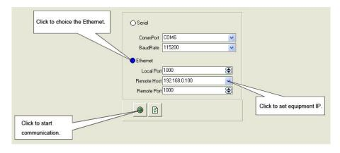
Ethernet, user can fill any number less than 1023 in local port, the remote port must be 192.168.0.100 and the remote port must be 1000. After setting above, click the icon to connect with the net work. If successful connect, the icon becomes, status on the left button showing
