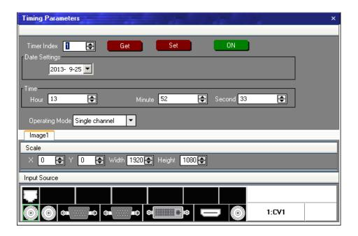
Timer Index: Timer index, currently, users can setup up to 10 timing operation in the schedule.
