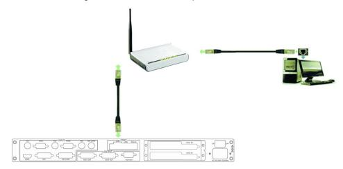
Step two: IP address setting (processor's default IP address is 192.168.0.100)
