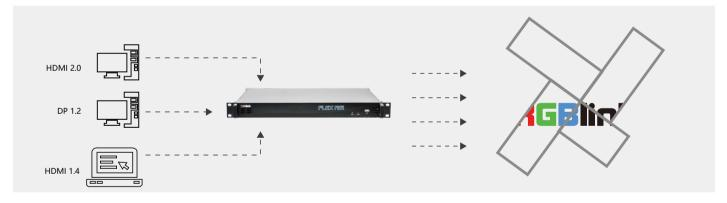
Each output can be configured independently allowing displays of multiple sizes and pixel densities to be supported
