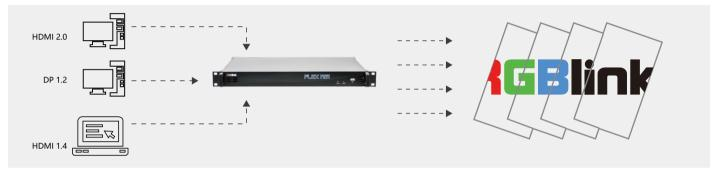
Overlapping displays are supported in any arrangement, opening up a wide range of application possibilities.
