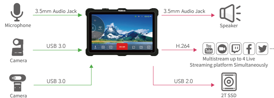
Scene 2: Seamless switching between different USB inputs
